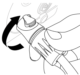
2 Rotate it by 15° until makes a click
